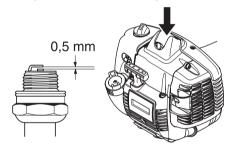
**CAUTION!** Always use the recommended spark plug type! Use of the wrong spark plug can damage the piston/cylinder.
